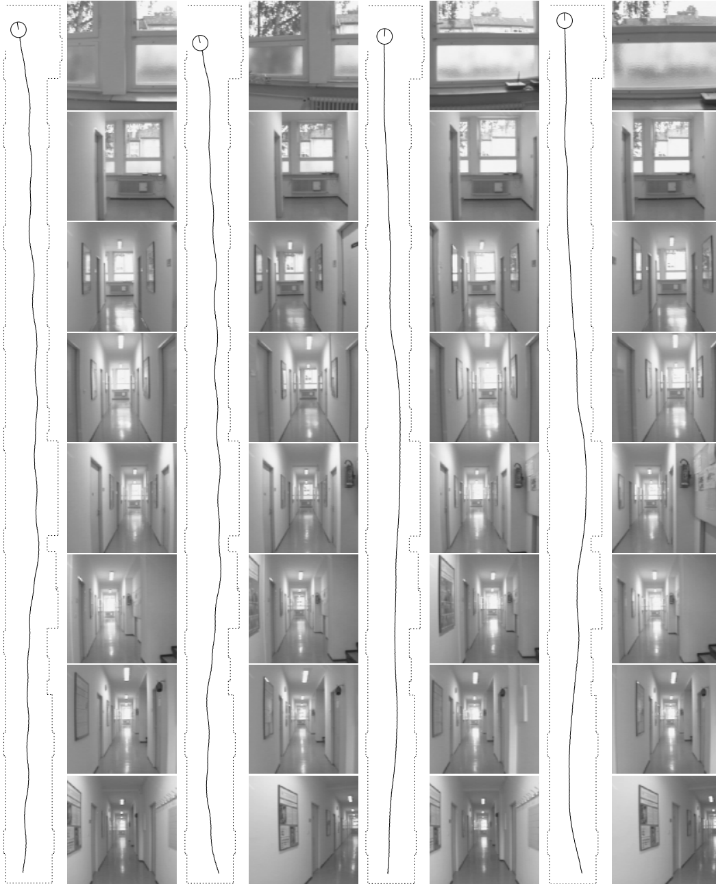
Figure 6. Path of the robot recorded from odometry data for different starting positions. The two on the left were recorded using the simple controller and the two on the right were recorded with the PID controller. The images along the path are a subset of the images that were recorded during execution of the algorithm. The path is overlaid on a map of the environment.
