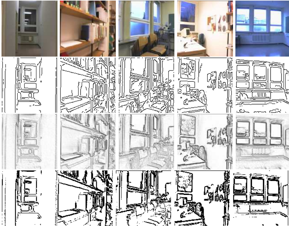
Figure 5: The first line of images show the set of images which were used to test the generalization capabilities of the detectors. The second line shows the output of the Canny edge detector. The third line shows the response of the best evolved edge detector. Finally the fourth line shows the binarized response of the best evolved edge detector with a manually set threshold of 0.25.
