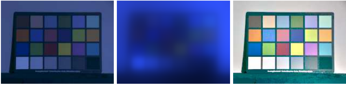
Figure 6: Results for the parallel algorithm on the image of the Macbeth color checker. The first image shows the input image. The second image shows local space average color. The third image shows the output image.
