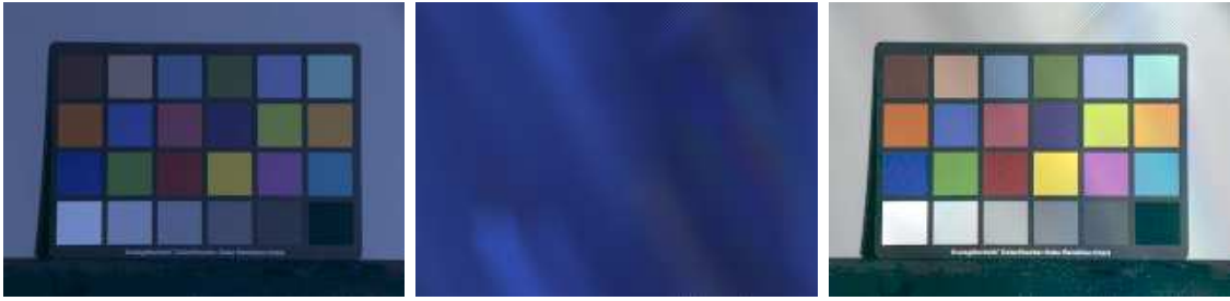
Figure 4: Results for a real image. The first image shows a Macbeth color checker taken from a database used to test color constancy algorithms. The database was put together by Barnard et al. [4]. The second image shows the estimated illuminant. The third image shows the output of the evolved individual.
