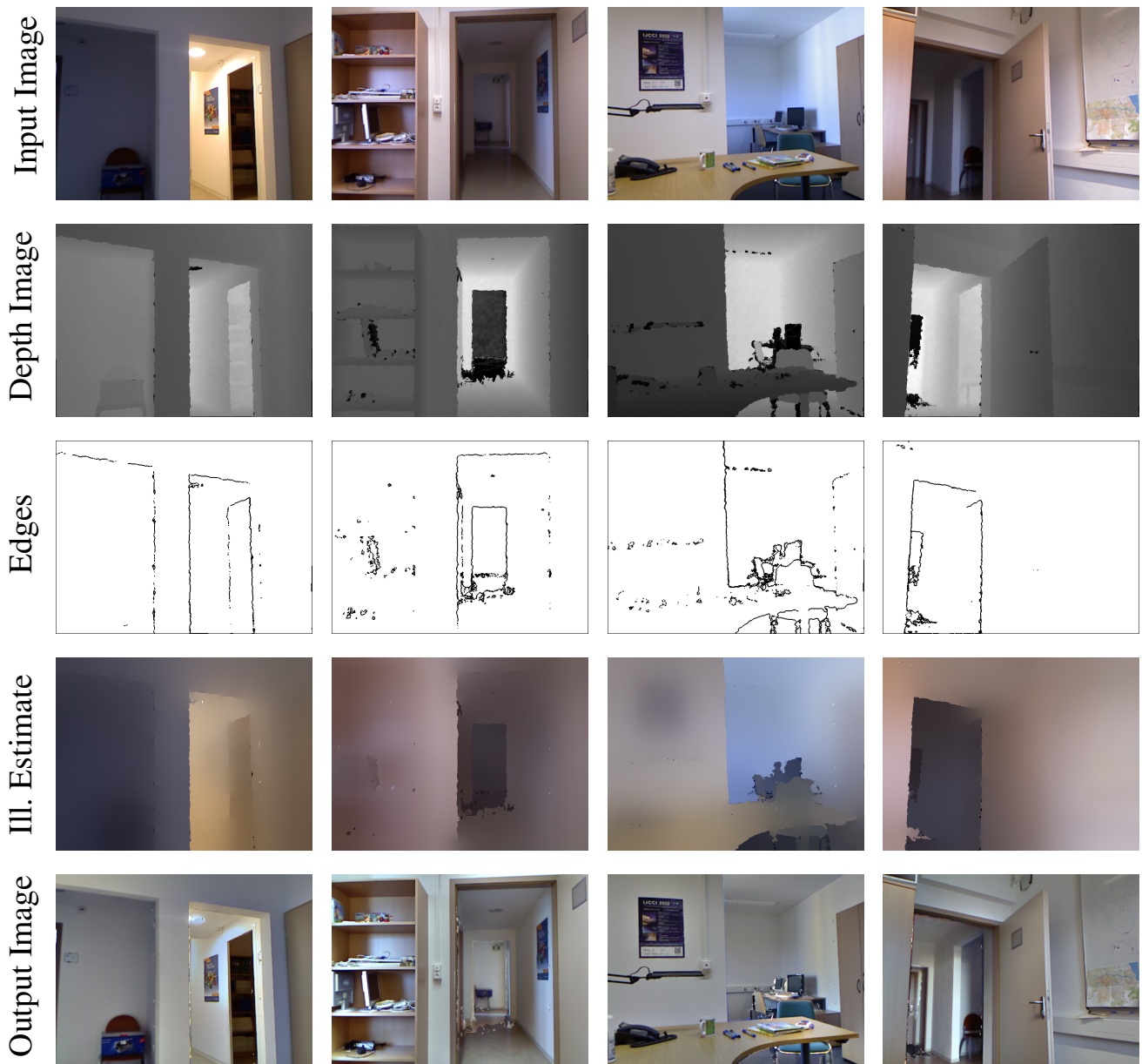
Fig. 6: Results for 4 sample images taken with the Kinect. From top to bottom, we have input image, depth map, detected edges, illuminant estimate and the computed output image.
