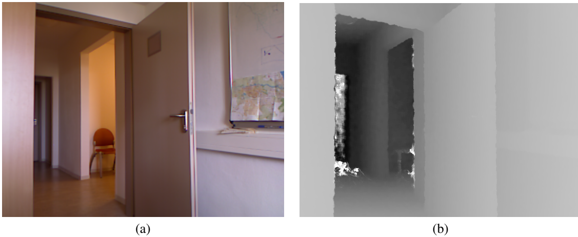
Fig. 16. (a) Visual perception of a scene. (b) Depth Map. Pixels that are closer to the camera appear brighter.
