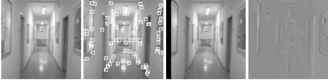
Figure 2: Image, image with sparse optical flow (after compensation for rotatory camera movement), previous image compensated for rotatory camera movement, difference picture between image and previous image compensated for rotatory camera movement.
