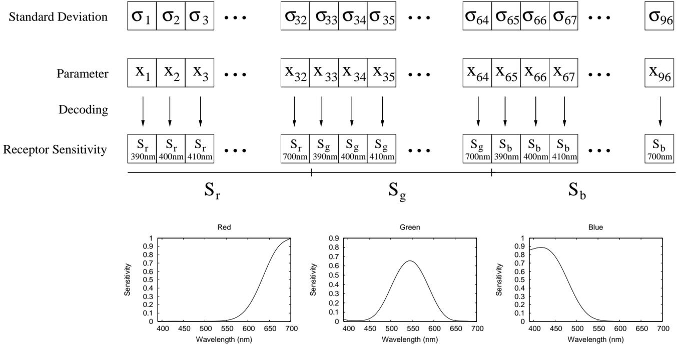
**Figure 3:** Each genotype represents three response curves for the three channels red, green, and blue. The genotype consists of 96 parameters  $x_i$  with  $i \in \{1, \dots, 96\}$  (32 per channel) and 96 standard deviations  $\sigma_i$ , which are used as mutation step sizes, i.e. we have a standard evolution strategy with automatic step size adaptation. Decoding of the individual is also shown. We have  $x_1 = S_r(390)$ ,  $x_2 = S_r(400)$ , ...,  $x_{96} = S_b(700)$ .
