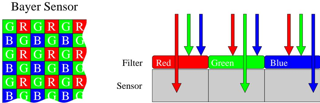
Figure 1: Bayer pattern (left). Filters are used to make the sensor respond in the red, green, and blue part of the spectrum (right).
