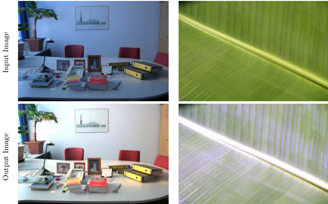
Fig. 1 Results using the gray world assumption for two different input images. The image on the left shows a typical office scene. The image on the right shows a leaf from a banana plant. The gray world assumption only works if there are a sufficiently large number of different colors in the scene.
