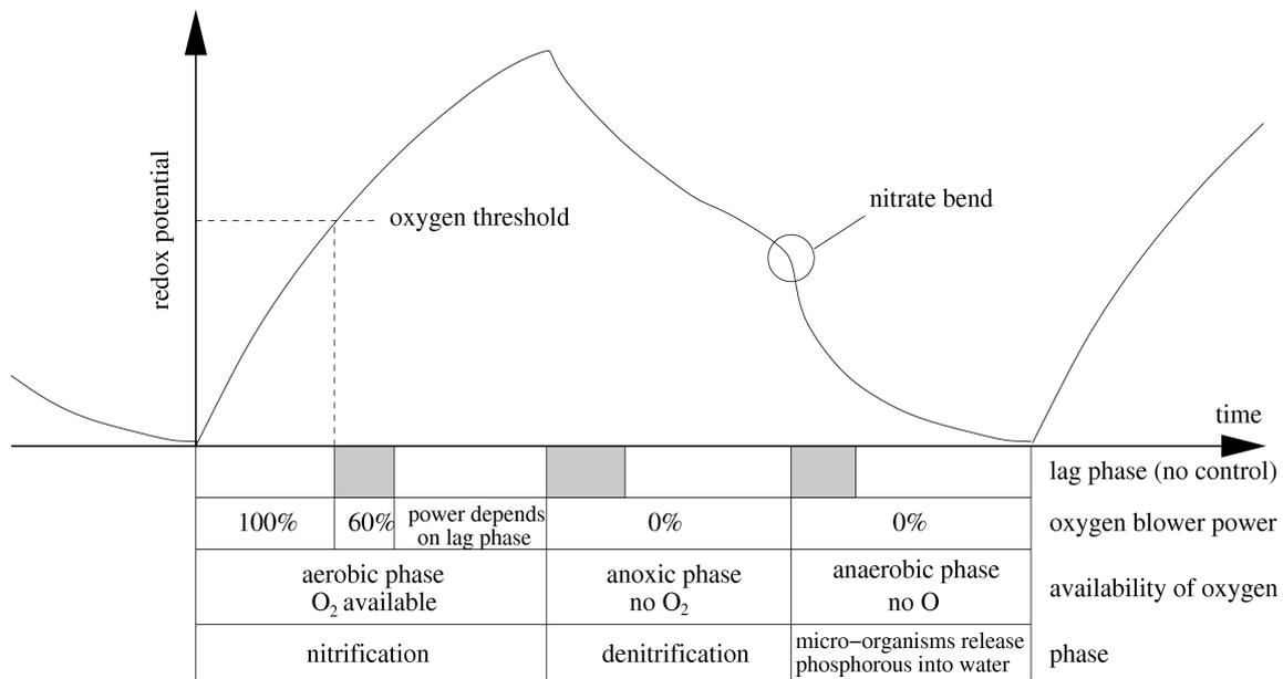
Figure 1: Idealized plot of the redox potential.
