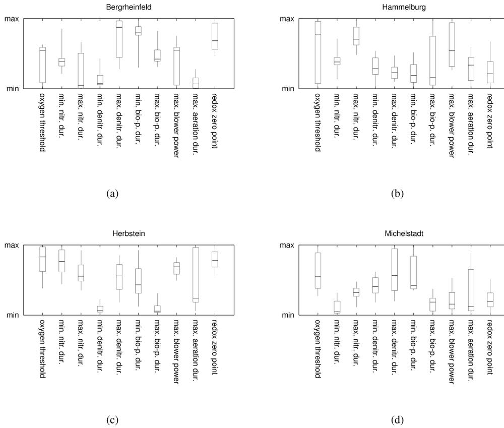
Figure 6: Box and whisker plots for the parameters of the non-dominated individuals found for plants (a) Bergrheinfeld (b) Hammelburg (c) Herbstein and (d) Michelstadt. Note that the scale for each parameter is given in Table 1.
