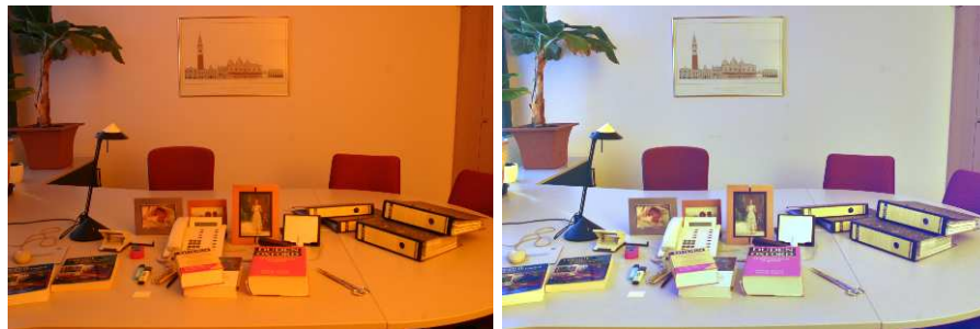
Fig. 1. The input image is shown on the left. Local space average color is computed using an exponential kernel. The output image is shown on the right.
